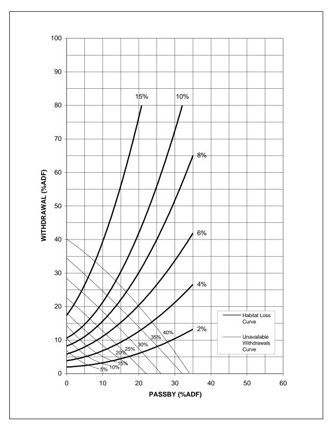
Figure 6.11. Impact of Selected Withdrawal and Passby Combinations, Unglaciated Plateau Segment Class 2 Streams, Wild Brook Trout
