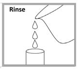
Rinse the sample cell with reagent grade water (distilled, deionized, or chlorine demand free water from lab) and then a small amount of primary standard solution
