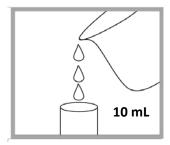
2. Fill sample cell with the calibration check standard to the 10 mL mark
