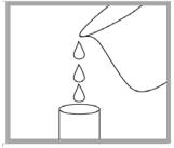
Rinse sample cell 2-3 times with reagent grade water (distilled, deionized, or chlorine demand free water from lab)
