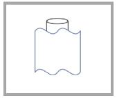
3. Wipe sample cell to remove fingerprints and moisture
