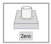
Place cell in meter, making sure to orient properly. Press "Zero" on meter to zero it out
