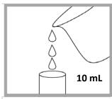
2. Fill sample cell with reagent grade water to the 10 mL mark
