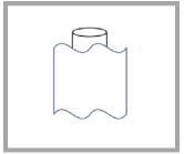
7. Wipe sample cell to remove fingerprints and moisture
