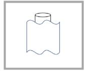
3. Wipe sample cell to remove fingerprints and moisture
