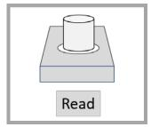
8. Properly orient sample cell and press "Read". Record the results in the "Measured Concentration" column of the form.
