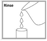
Rinse the sample cell with reagent grade water (distilled, deionized, or chlorine demand free water from lab) and then a small amount of primary standard solution
