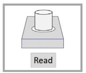
8. Properly orient sample cell and press "Read". Record value as the Method Blank on form.\*
