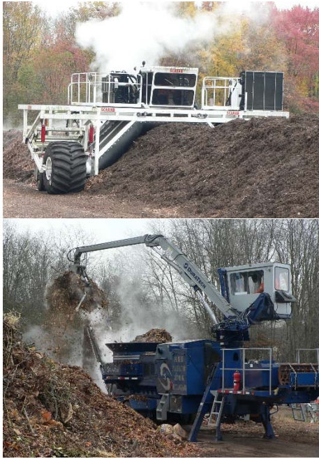
Top: A straddle turner turns compost. Compost is turned periodically until it is mature.
