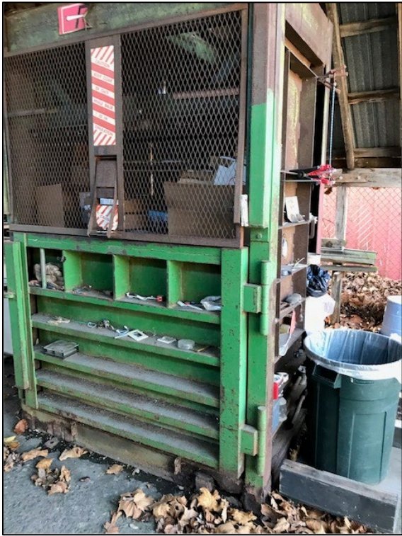
Vertical baler for processing select materials
