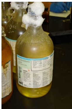
Example of a leaking container
