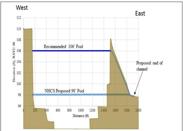
Figure 2 – Comparison of Profile with Pool level at Elevation 106' to NHCS Proposed Pool and Discharge at Elevation 98'. [Source: NHCS Bonding and Reclamation Map 4/12/2016, Vertical Exaggeration: 10:1]
