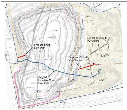
**Figure 1:** Comparison of original Primrose Creek flow path and NHCS proposed flow paths into and out of the quarry pit. [Proposed flow path from ERG, NHCS Bonding and Reclamation Map 4/12/2016, Previous Primrose Creek from NHCS Mining Plan April 1974]
