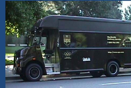
Workhorse W42 Chassis step-van chassis w GM 4.8L engine, and Workhorse W62 with GM 6.0L engine; FCCC MT45 chassis with GM 6.0L (soon)
