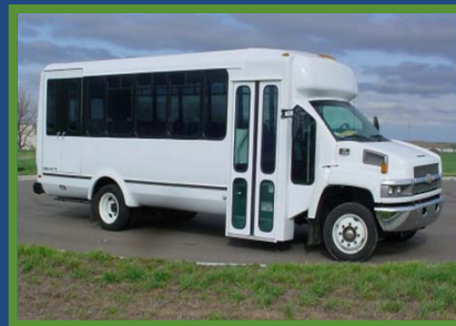
GMC C4500/5500 Series Cutaway w 8.1L GM engine (retrofits of existing stock only)
