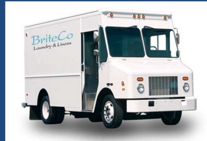
Workhorse W42 Chassis step-van chassis w GM 4.8L engine, and Workhorse W62 with GM 6.0L engine; FCCC MT45 chassis with GM 6.0L (soon)
