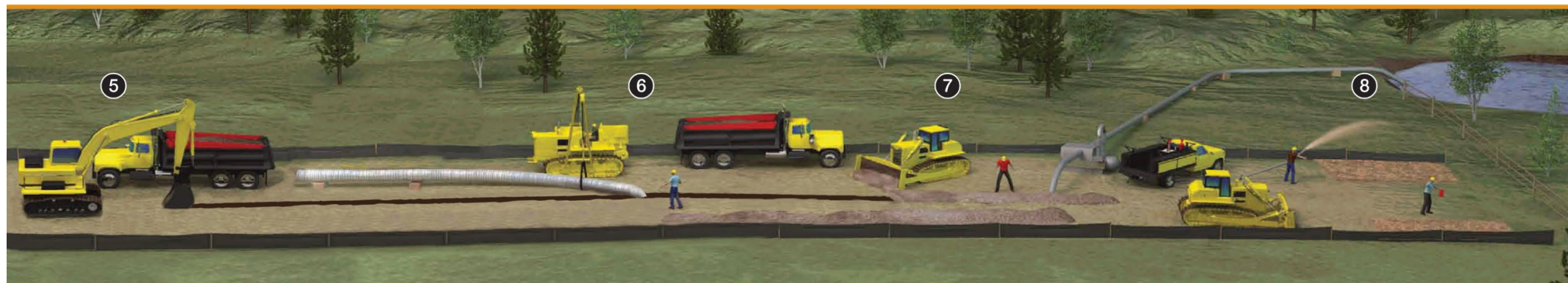
Figure 1.3-1 Typical Pipeline Construction Sequence
