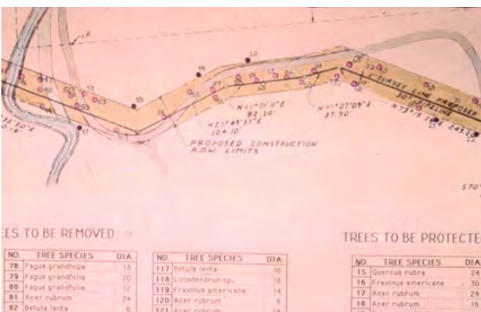
Construction documents detailing trees to be removed as well as trees to be saved, L. Sauer
