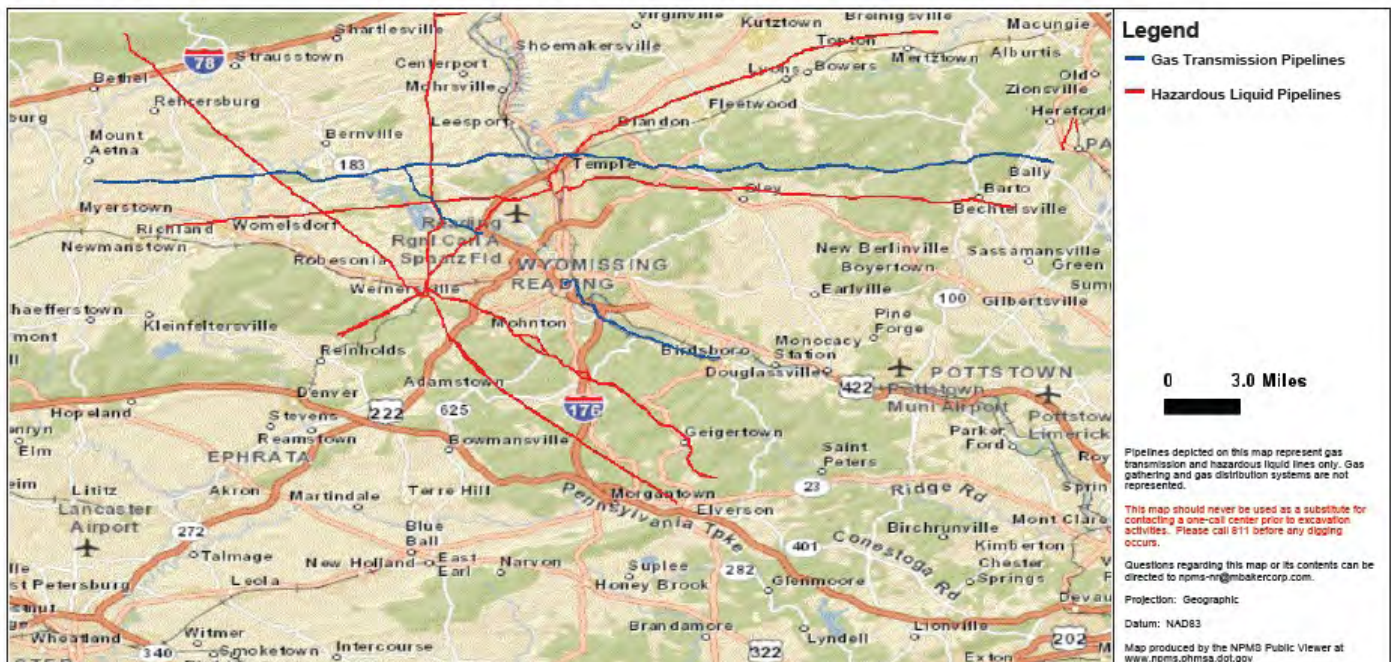
A map of the Reading, PA, area created using the National Pipeline Mapping System (NPMS) Public Map Viewer online. Users can view NPMS data one county at a time. The pipelines shown include gas transmission pipelines (blue) and hazardous liquid trunklines (red). Data for gathering or distribution pipelines is not available through the NPMS Public Map Viewer.
