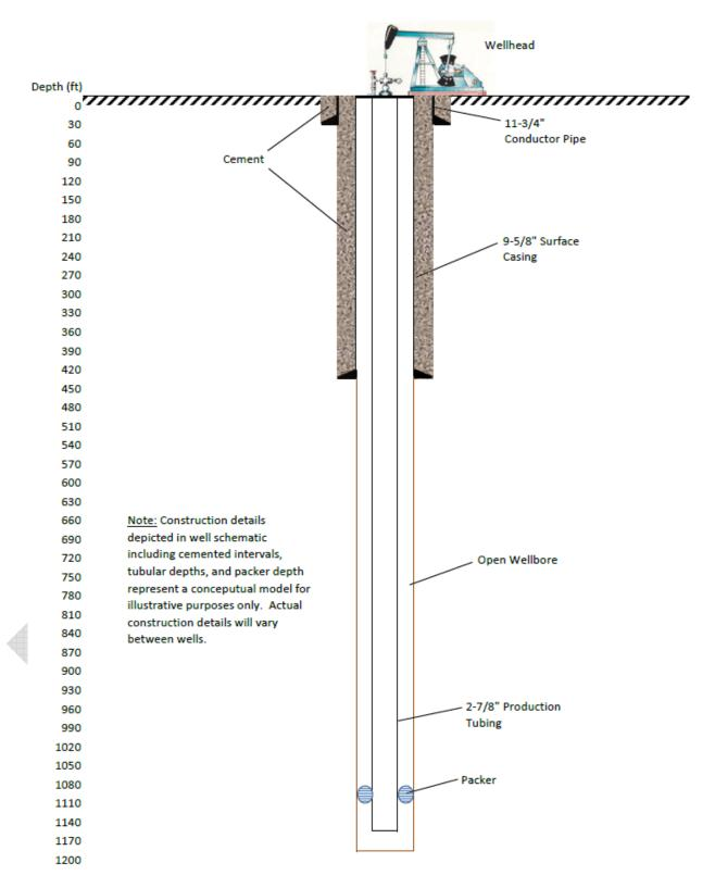
Schematic representing example of oil well where water level measurement may be appropriate
