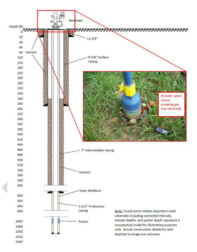
Schematic representing example of gas well not fitted for annular space pressure monitoring
