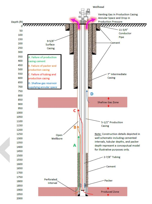
Schematic representing mechanical integrity failures and well construction flaws that would generate open flow in annular space of production casing
