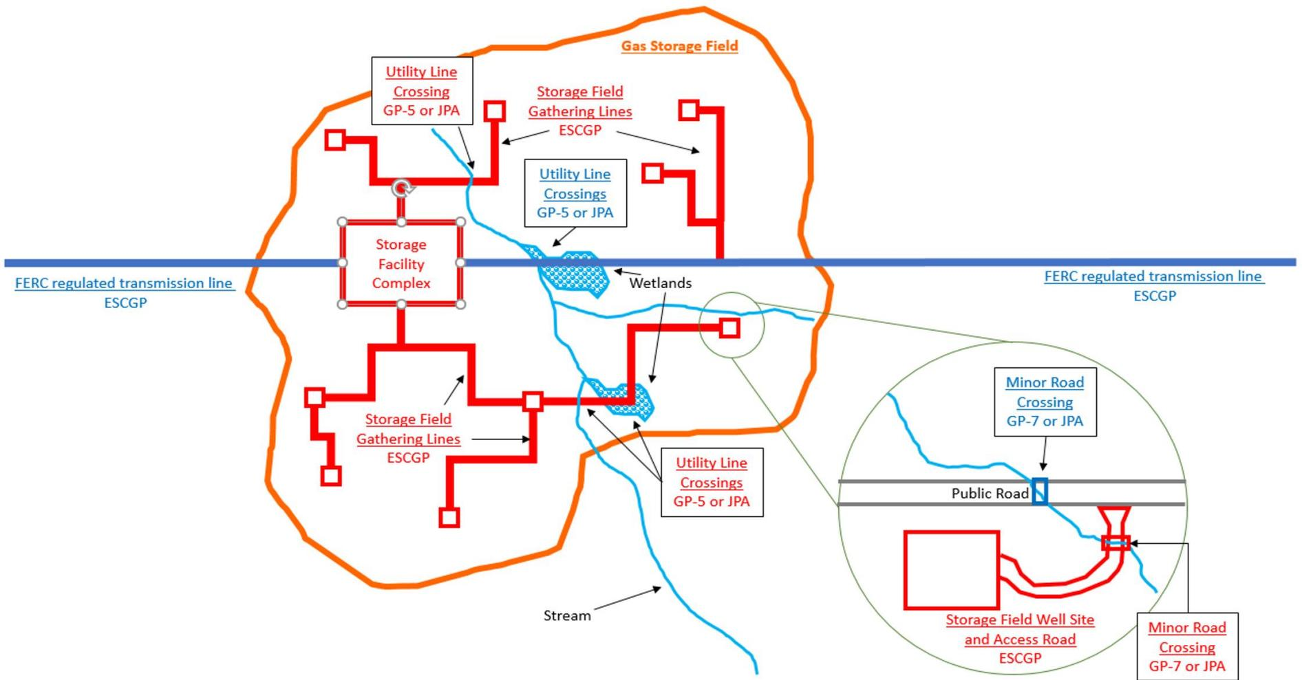
Figure 2: Illustration of gas storage fields
