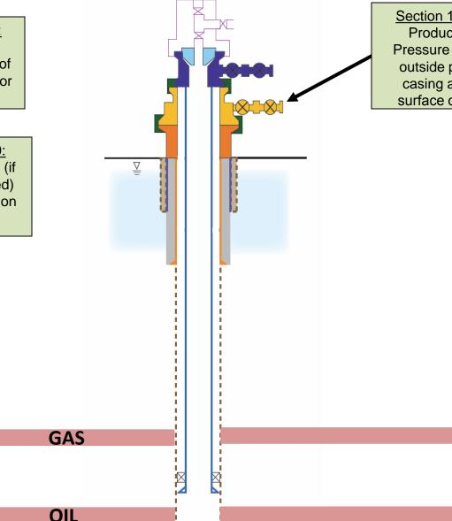
Section 13: Annular Production Gas Pressure (measured outside production casing and inside surface casing "P")
