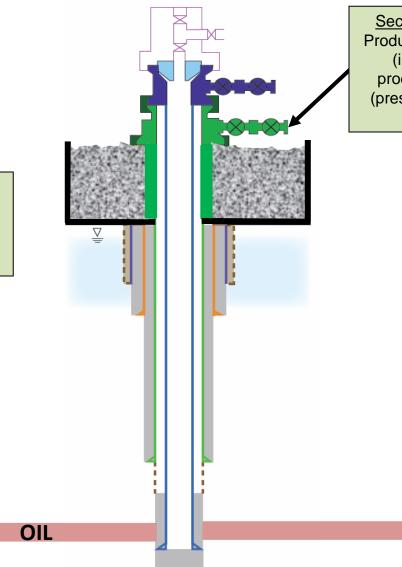
Section 14: Primary Production Annulus "P" (intermediate x production) Shut-in (pressure) or Venting (Flow Rate)
