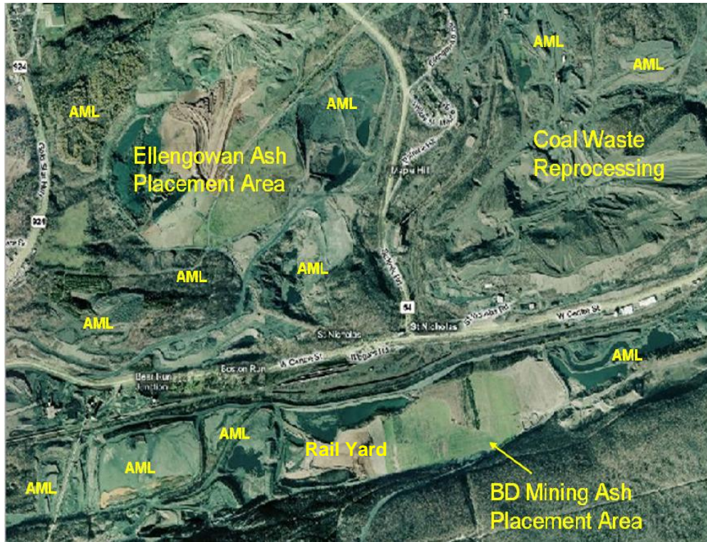
Figure 4. BD Mining area. AML indicates some of the abandoned mine features. The Coal Waste from the area just north of BD Mining is going to the Schuylkill Energy site and the ash is being placed at the Ellengowan site. BD Mining's ash is coming from the Gilberton power plant, which is south of the area shown. The revegetated (green) areas are the reclaimed areas where ash was placed. (Image from MSN Live Search Maps)
