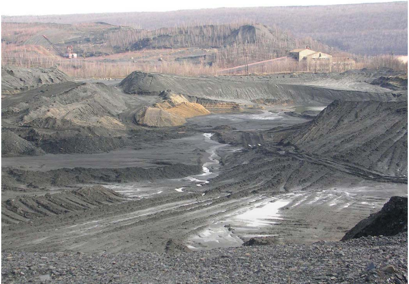
Figure 2. The area pictured is just to the north of BD Mining. Everything in this picture, with the exception of the hill in the distance (and to some extent, it too) is abandoned mine lands. Most of the material that can be seen is waste coal. This waste coal is being used to fuel local fluidized bed combustion power plants. The building in the upper right is the abandoned St. Nicholas coal breaker.
