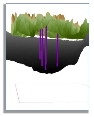
The point layer is "draped" over a surface elevation raster. Z-values are added to the points' geometry.
