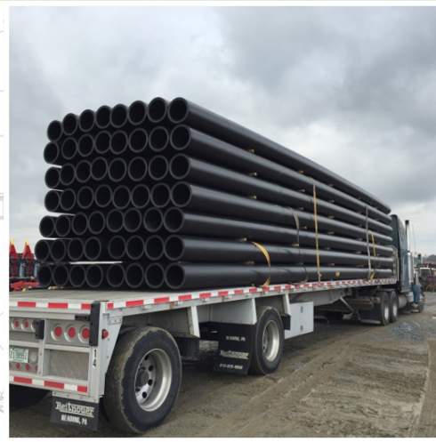
Truck carrying high-density polyethylene (HDPE) pipe used for waterline mains
