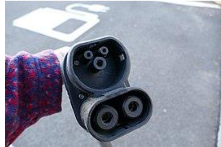
Level 3 (DCFC) charger head CCS
